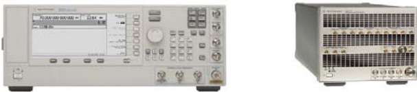
Figure 3. Agilent™ 8257 and N8211 Synthesizers supported as auxiliary RF signal sources in the SMART^E™ environment.
